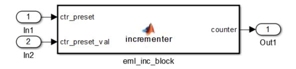
The root-level model drives the subsystem and includes Display and To Workspace blocks for use in simulation. (The Display and To Workspace blocks do not generate HDL code.)
