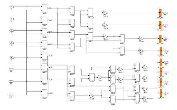
Set **DistributedPipelining** to **on** and **OutputPipeline** to **6** to distribute 6 pipeline stages for each signal path in the DUT.
