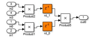
Now, use constrained output pipelining to further reduce the critical path.
