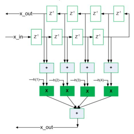
The following figure shows the sharing architecture automatically implemented by HDL Coder when the sharing optimization option is turned on.
