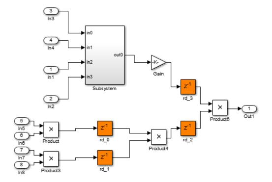
The subsystem now contains pipeline registers:
