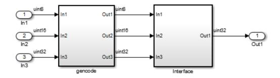
Suppose that you want to generate HDL code from top, with a black box interface from the Interface subsystem. To specify a black box interface:
