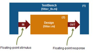
For floating-point to fixed-point conversion, the following requirements apply to the original design and the testbench:
