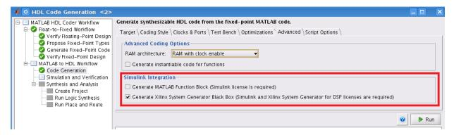
To generate code compatible with a Xilinx System Generator Black Box, set:
