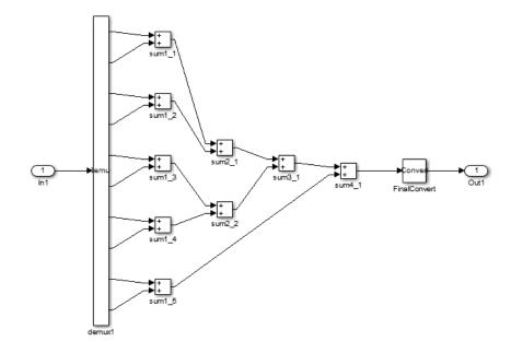
The generated model implements the vector sum as a tree of adders (Sum blocks). The vector input signal is demultiplexed and connected, as five pairs of operands, to the five leftmost adders. The widths of the adder outputs increase from left to right, as required to avoid overflow in computing intermediate results.
