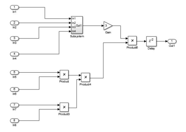
The following diagram shows the model after distributed pipelining redistributes the delay to reduce the critical path.
