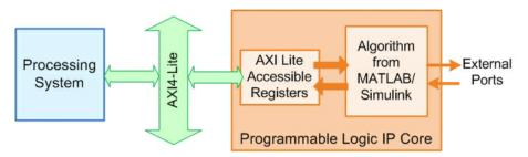
This IP core also support the **External Port** interface. To connect the external ports to the FPGA external IO pins, add FPGA pin assignment constraints in the Xilinx EDK environment.
