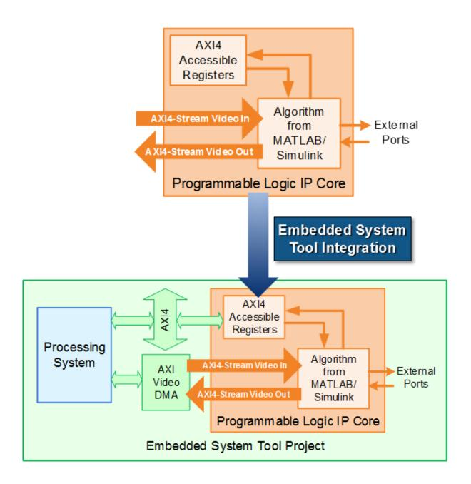
**4** *SW Interface Model Generation* (requires a Simulink license and Embedded Coder license): In the HDL Workflow Advisor, after you generate the IP core and insert it into the reference design, you can optionally generate a software interface model. The software interface model is your original model with AXI driver blocks replacing the hardware part.
