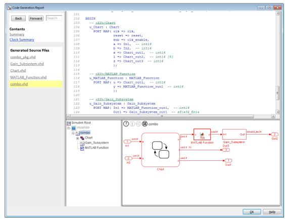
**6** Click a link in the code. The model Web view displays and highlights the corresponding block in the model.
