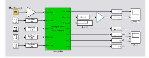
The model contains the Simulink Real-Time interface subsystem. This new subsystem replaces the DUT (ServoSystem) in the original model. It replaces the internals of the original DUT with a Simulink Real-Time FPGA block and other blocks to work with the algorithm on the FPGA.
