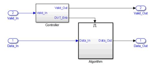
As another example, you can use a controller in your DUT that generates an enable signal for the enabled subsystem.
