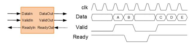
For example, if you have a FIFO in your DUT to store a frame of data, you can model the Ready signal based on the FIFO Full signal to apply back pressure to the upstream component.
