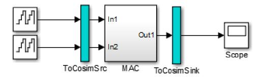
The two subsystems labelled ToCosimSrc and ToCosimSink do not change the performance of the simulation path. Their purpose is to capture stimulus and response signals of the DUT and route them to and from the HDL cosimulation block (see "Signal Routing Between Simulation and Cosimulation Paths" on page 18-46).
