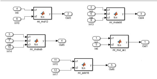
For example, the ml\_mul\_acc MATLAB Function block shows how to write a multiplyaccumulate operation in MATLAB. "Use the hdlfimath Utility for Optimized FIMATH Settings" on page 20-36 applies fixed-point math settings that are appropriate for HDL code generation.
