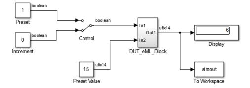
You might want to experiment with the results of toggling the Control switch, changing the Preset Value constant, and changing the total simulation time. You might also want to examine the workspace variable simout, which is bound to the To Workspace block.
