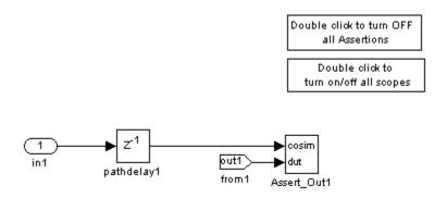
To verify that a generated model with streaming is bit-true to its original counterpart in a validation model:
