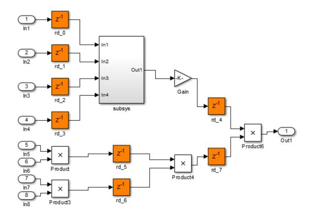
In the **subsys** block, there are no delay blocks because hierarchical distributed pipelining is not enabled.
