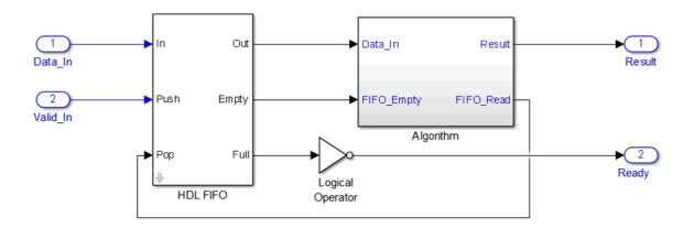
**Note:** If you have delay balancing enabled, the software can insert one or more delays on the Ready signal. Disable delay balancing for the Ready signal path.
