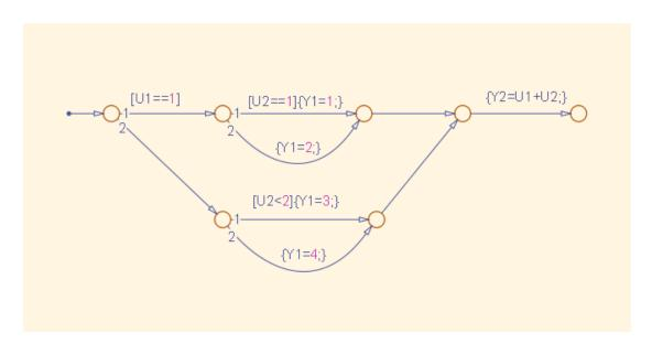
The following generated VHDL code excerpt shows the nested IF-ELSE statements obtained from the flow diagram.
